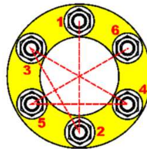
Criss-Cross Tightening Sequence for Circular Bolt Patterns
